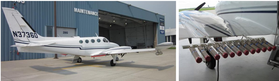
Figure 5: Image showing the Cessna 340 aircraft used during POLCAST2 and the end of POLCAST3 located at the Fargo Jet Center in Fargo, North Dakota. Shown on the right is an image of one wing with a full set of hygroscopic flares. Both images were taken during POLCAST3.
